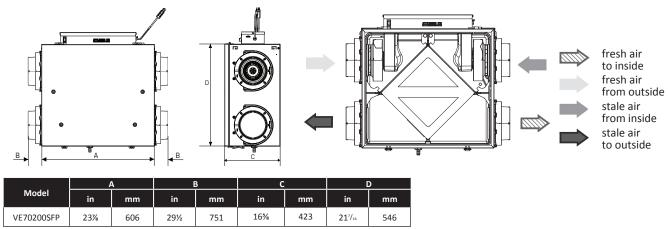
Clearance of 22" (559 mm) in front of the unit is recommended for removal of core. All units feature three foot plug-in power cord with 3-prong plug.
